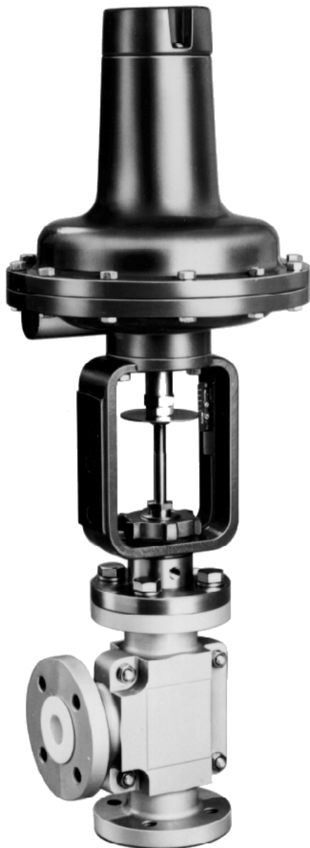
1" – Model "520" Control Valve with Air-to-Open, Fail Close Model 30R Actuator.
