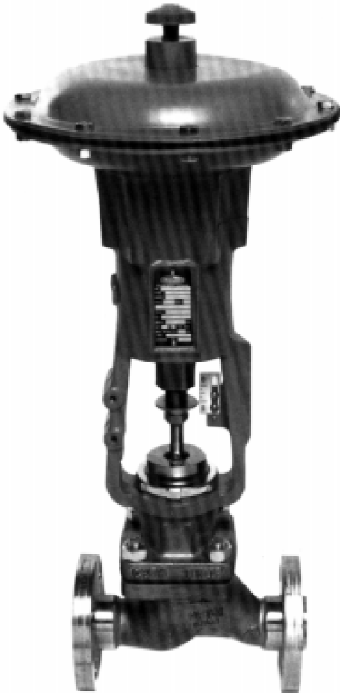
Model 989 1" – Body Size CF3M Body – 300# Flanged Model 55R Actuator (ATO-FC Action) "Short Pattern"
